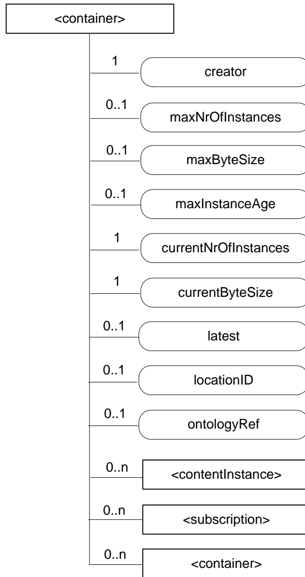
Figure 9.6.6-1: Structure of <container> resource
