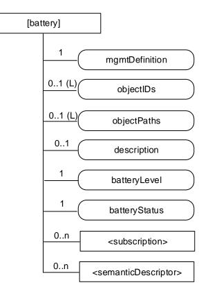
Figure D.7-1: Structure of [battery] resource
