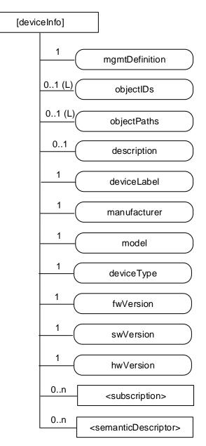
Figure D.8-1: Structure of [deviceInfo] resource
