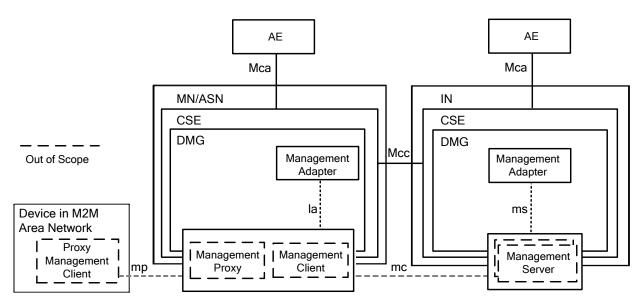
Figure 6.2.4.1.1-1: Device Management Architecture
