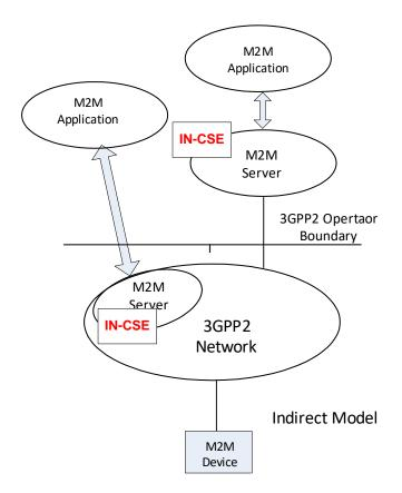
Figure C.2-2: Multiple M2M Applications Using Diverse Communication Models
