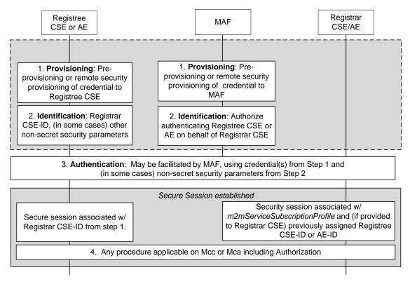
Figure 11.3.0-2: MAF assisted High Level Procedures on Mcc or Mca
