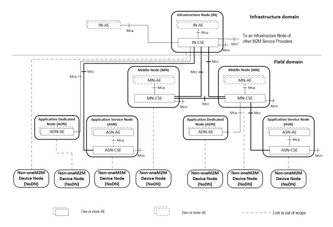
Figure 6.1-1: Configurations supported by oneM2M Architecture
