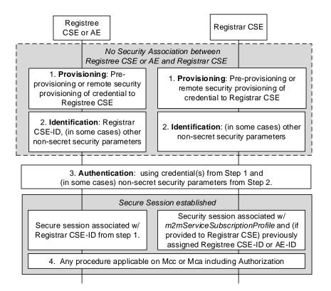
Figure 11.3.0-1: High Level Procedures on Mcc or Mca without MAF
