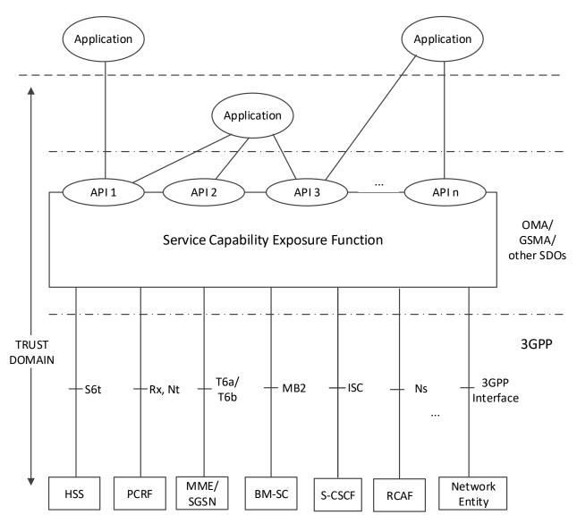
Figure B.2.2.1-2: 3GPP Architecture for Service Capability Exposure
