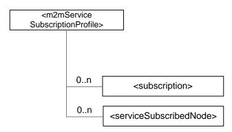
Figure 9.6.19-1: Structure of <m2mServiceSubscriptionProfile> resource
