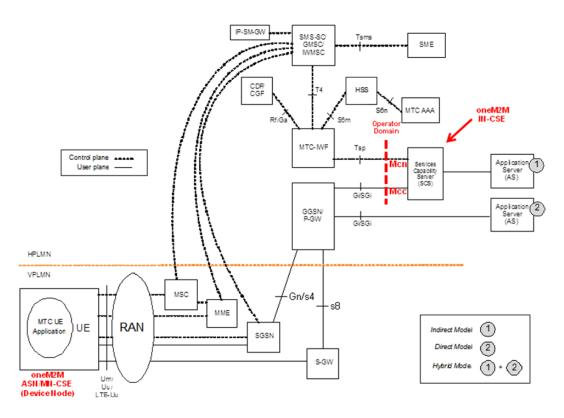
Figure B.2.1-2: Mapping of oneM2M entities to the 3GPP Architecture for Machine-to-Machine Communications
