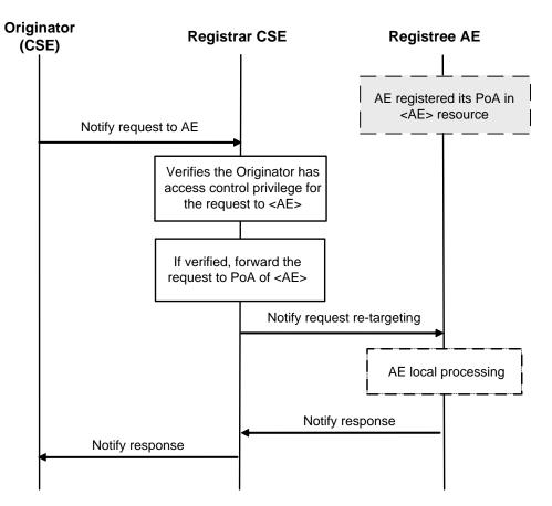
Figure 9.3.2.3.1-1: Re-targeting a notification request to an AE
