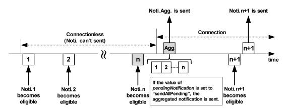
Figure 10.2.12.1-2: Notification Mechanism when pendingNotification (sendAllPending) is used
