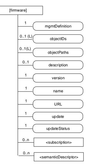
Figure D.2-1: Structure of [firmware] resource
