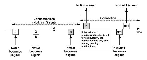
Figure 10.2.12.1-1: Notification Mechanism when pendingNotification (sendLatest) is used
