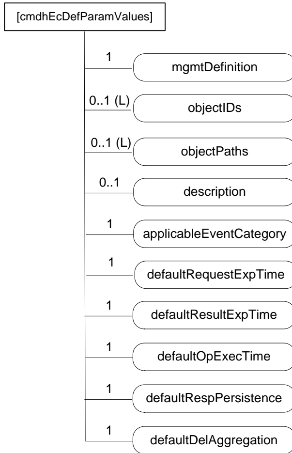
Figure D.12.4-1: Structure of [cmdhEcDefParamValues] resource
