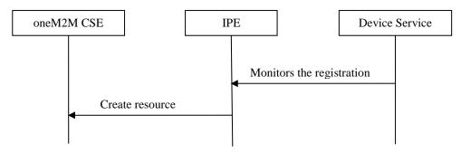
Figure 6.4-1: Procedure of registering Device service
