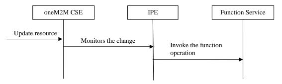
Figure 6.5-3: Procedure of invoking function operation
