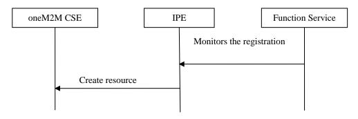
Figure 6.5-1: Procedure of registering function service
