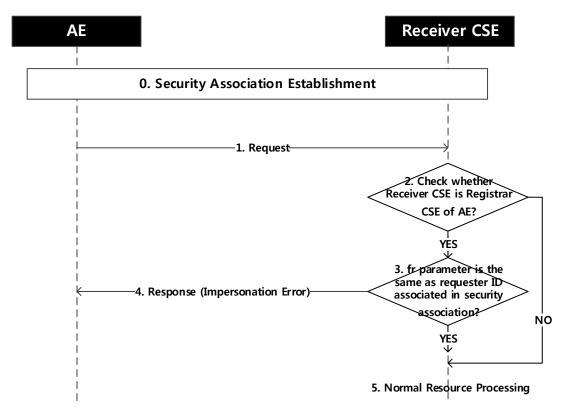
Figure 7.2-1: AE impersonation checking procedure
