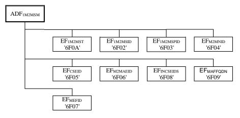
Figure D.2: File identifiers and directory structures of ADF<sub>1M2MSM</sub>
