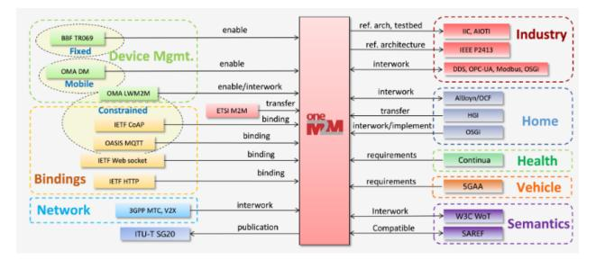
Figure 6 oneM2M unites established standards and addresses emerging use-case requirements
