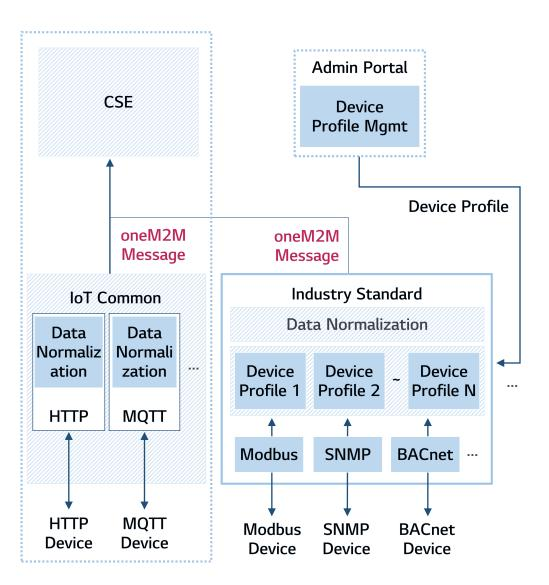
Supports widely used protocols for IoT: HTTP, MQTT, CoAP and WebSocket
