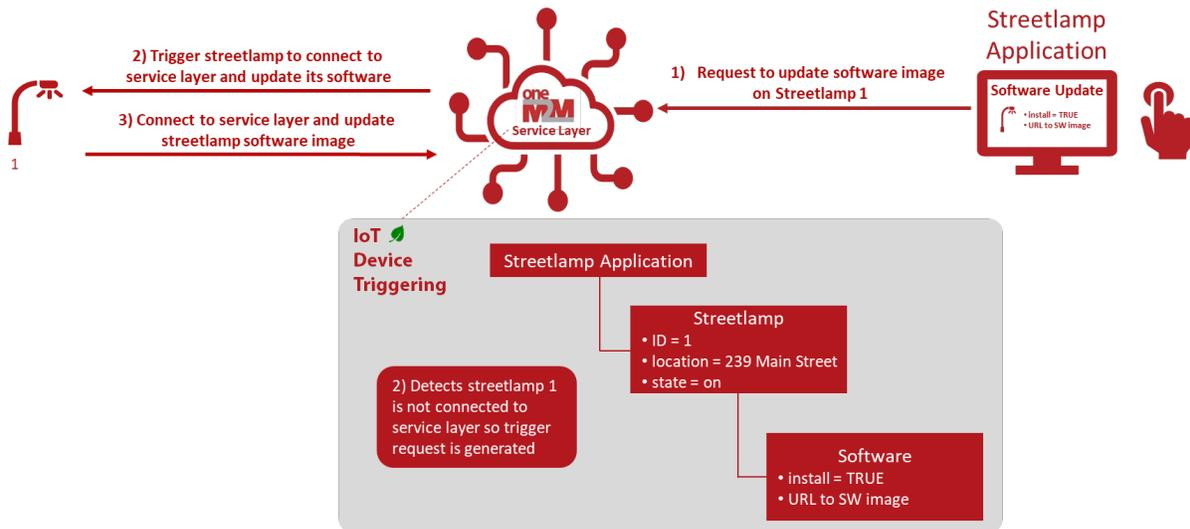
Figure 4 - oneM2M Device Triggering Feature
